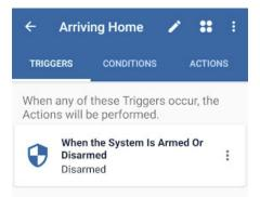
This scene will unlock the front door and turn on the living room lights (action) when the system is disarmed (trigger) when it is between sunset and sunrise (condition).
